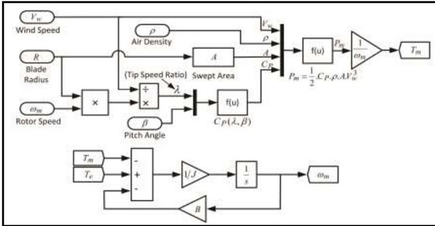
**Fig. 1.** Dynamic model of wind turbine [7].
